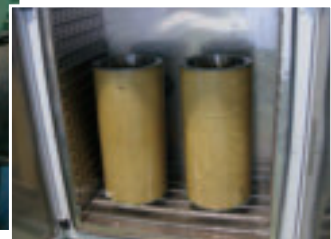
Bonded joint curing
